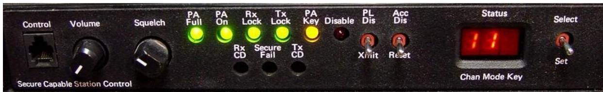
Photograph of a digital-capable station transmitting on channel 1, mode 1.
