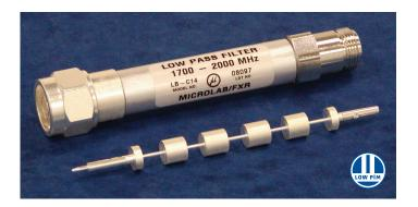
Microlab Model LB series low pass filters are designed to suppress harmonics and out of band noise and interference, to improve signal quality in high power system applications and bench testing.
