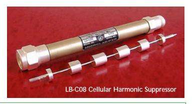
Microlab/FXR Models LB-C07/CO8/C14 are designed to suppress the harmonics of the transmitted base station signal. These harmonics are often generated in the final isolator.
