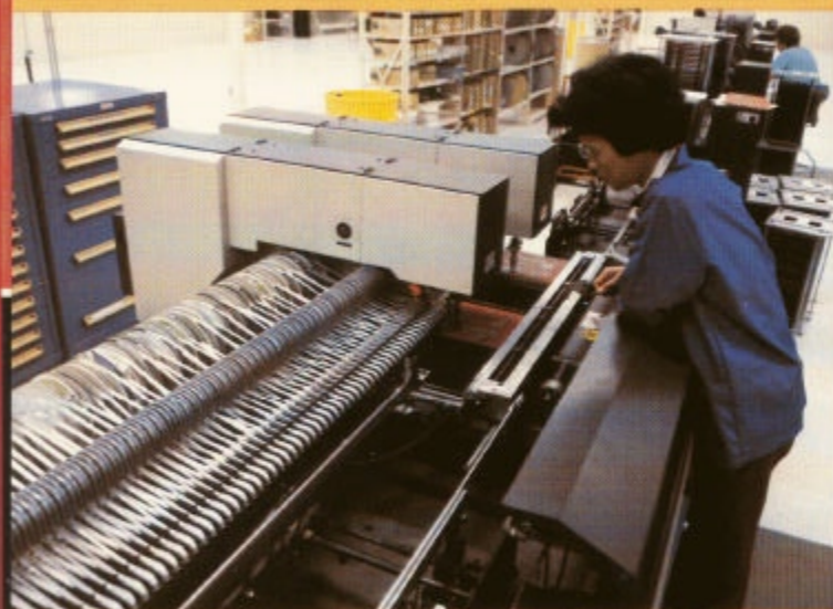
High speed, computer controlled auto insertion of printed circuit boards
