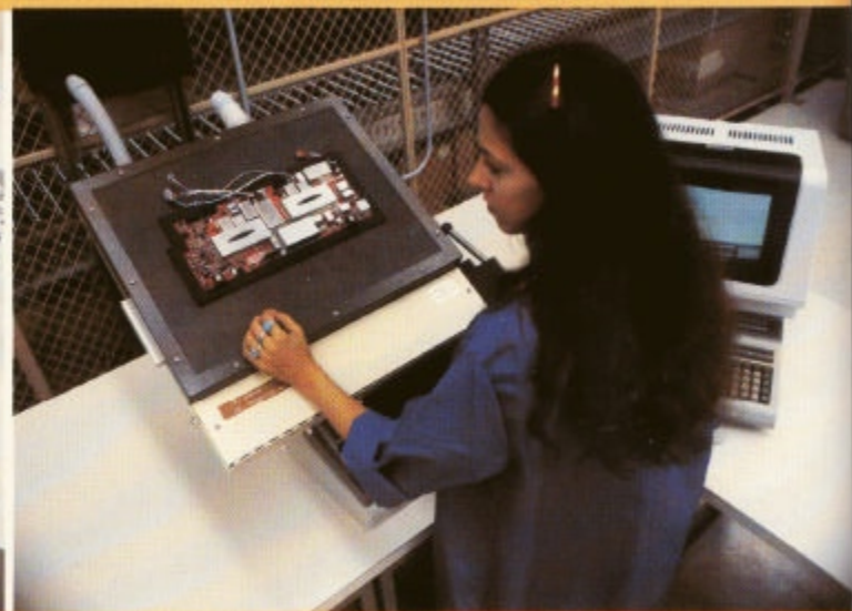
Computerized board testing of the RF circuit board
