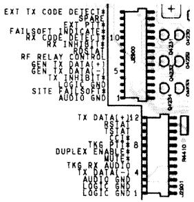
Most of the pins used for the interface to the RC-850 are available from the MRTI connector (see above). However, one pin that is required but not available on that connector is some sort of Carrier On Receive (COR) signal.
